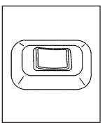
Your vehicle may have this feature. The driver's and passenger's seatback lumbar support can be adjusted by moving the control located on the outboard side of the seat cushions. To increase or decrease support, hold the control forward or rearward. Keep in mind that as your seating position changes, as it may during long trips, so should the position of your lumbar support. Adjust the seat as needed.
